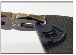
Insert a second T-nut through the clip and into the top side of the right half of your board nose. Press the T-nut using pliers as straight as possible without turning.
