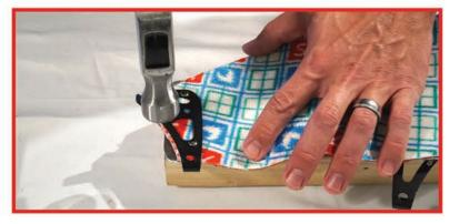
Place the zip strip tail on the wood block. Use the included punch with your hammer to make four holes in the zip strip on the marks.
