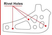
Fold skin in half leaving the front 2 inches (5cm) exposed. Stick the zip loc bag that this kit came in onto the exposed glue on the back of the skins to protect it. Hammer the nail just through the tip of the skin into the three dots using a wood block as a backer. Be sure to push the nail all the way through the holes by hand to insure the correct hole size.
