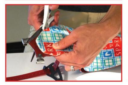
Remove the tipclip and align the plastic slip plate with the rivet marks. Trace the front edge of the slip plate. If the line doesn't go all the way across the skin, continue drawing the line down to transition into the existing skin curve. Pro tip: place your other skin on top and use that curve as a guide. Cut off the excess fabric.
